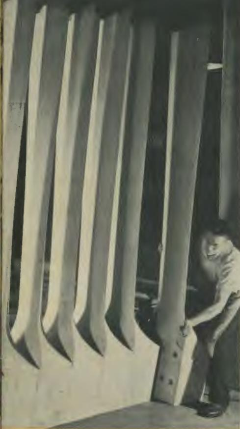
Sitka spruce is a unique wood with a multitude of specialized uses. It is used for propellers in all large wind tunnels and provides virtually all piano sounding boards produced in this country.
